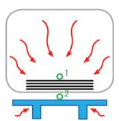
This lag also results in the addition of wasted energy to the system while the surroundings heat up and the heat eventually soaks into the part.
