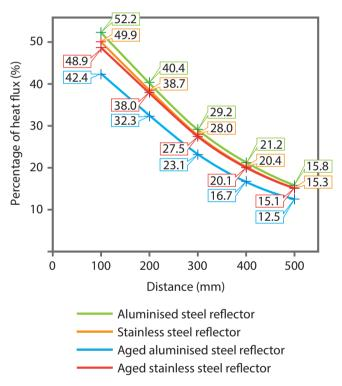
Percentage of heat flux as a function of distance from element
