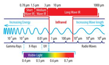
Infrared is substantially different to conduction and convection. As we all know, radiation doesn't need a medium to travel in – it's how the sun heats the earth; however the key issue that consistently gets 'lost in translation' is that IR is a form of energy, not heat. So what happens when this energy is incident on a surface? Similar to visible light, what we see is three processes occurring: reflection, transmission and absorption.
